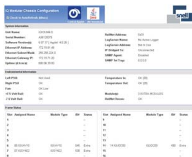
IQH3B Http based frame status overview
