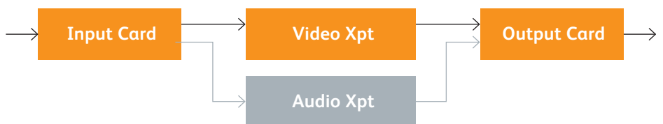
All input and output card positions have connections to video and audio crosspoints
