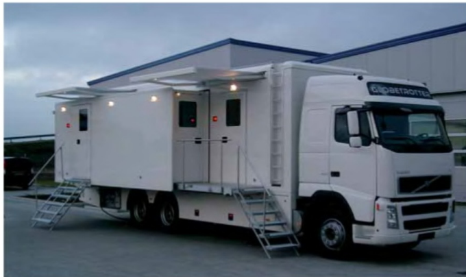
Designed to operate in the 1080/50i HD format, SZMG's new OB vehicle processes feeds from eight HD camera sources with the capability to expand to a 14-camera operation through linkage with an electronic field production system.
