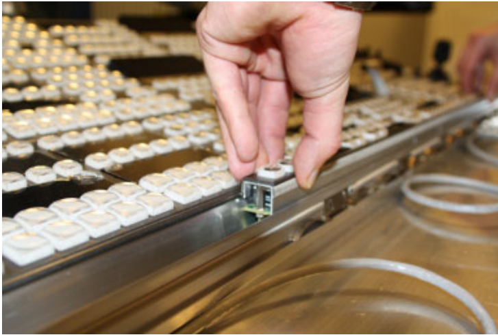
Aligning the System Bar for Replacement
